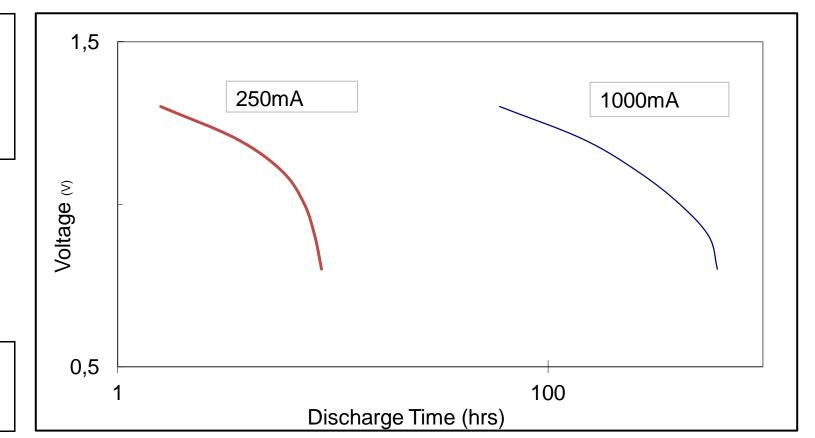
Test environment: 20  $^{\circ}$ C  $\pm$ 2,60%  $\pm$ 15% R.H, Load resistance: 3.9 ohms, time: 0.3s
